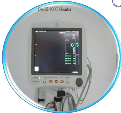
DASH® 4000 Monitor For continuous cardiac monitoring (Vitals, ECG, O2 saturation etc.)
